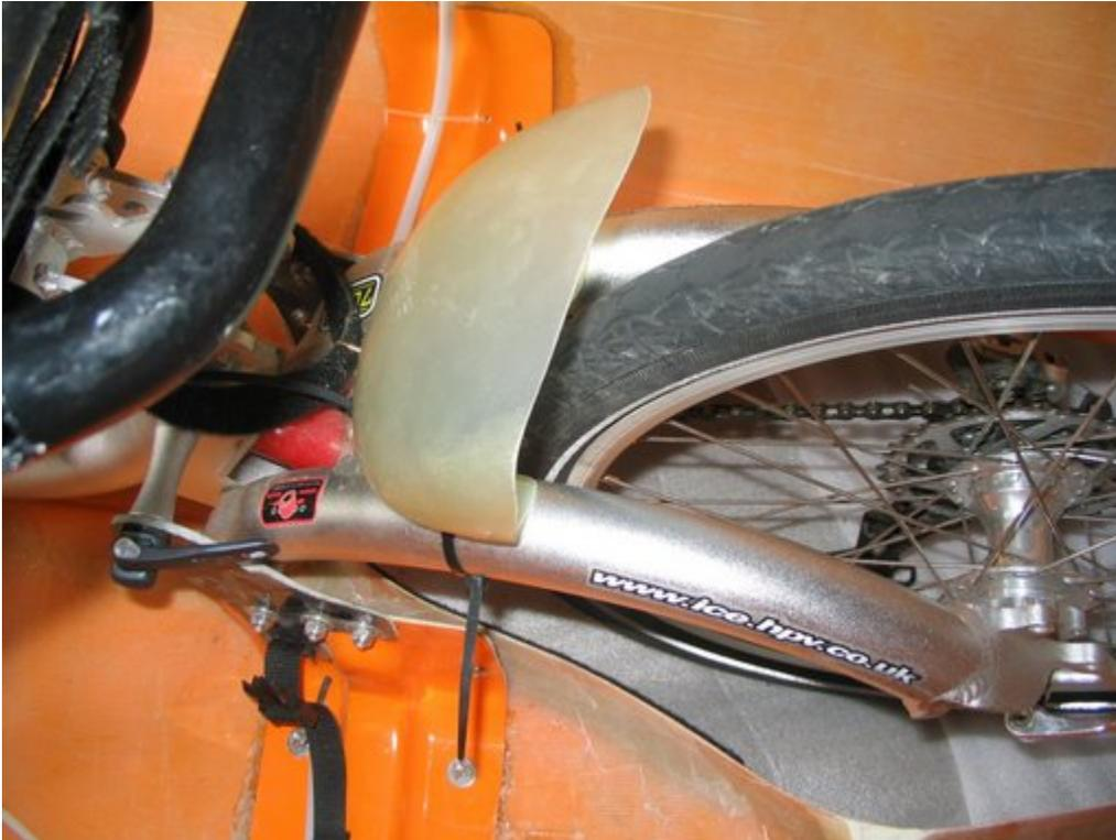
Before attaching the rear fender install the strap assembly to the swing arm. First roll up the Velcro that normally holds the swing arm up when you lift the back on the trike. If you don't plan on taking the trike out of the shell in the future you can remove this whole part. Now thread the red strap in place as per picture.
