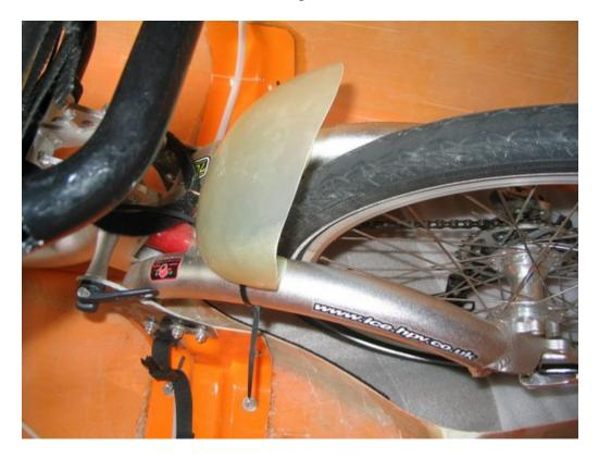
Before attaching the rear fender install the strap assembly to the swing arm. First roll up the Velrco that normally holds the swing arm up when you lift the back on the trike. If you don't plan on taking the trike out of the shell in the future you can remove this whole part. Now thread the red strap in place as per picture.
