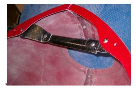
The next step is to add the back bottom section to the front section. They are held together with 10-24 truss head bolts. The bolt goes in with the washer and the nylock nut on the inside.
